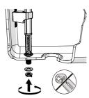
11. Install the fill valve into tank, rotate the gasket and
