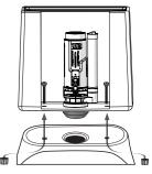
6. Take the water tank and install it on the two piece toilet of mounting holes, then fasten the bolts.
