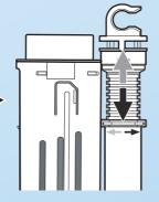
Adjust it to be 45mm higher than the water level when the horizontal cross-section is smaller than 300cm<sup>2</sup>. (ACCORDING TO ISRAEL STANDARD)
