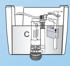
Connect the tube to the back of water tank.
