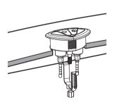
Insert Button Body in the button hole of lid and separately level the Full Flush Button and Partial Flush Button of Push Button at those of Flush Valve, then load U Buckle into Button Body(as picture) and screw Fix Nut to U Buckle tightly.
