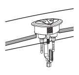
Insert Button Body in the button hole of lid and separately level the Full Flush Button and Partial Flush Button of Push Button at those of Flush Valve, then load U Buckle into Button Body( as picture) and screw Fix Nut to U Buckle tightly.
