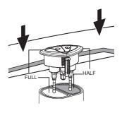
Loose Eight-square Nut and adjust the height of Rod to expected, then screw Eight-square Nut tightly.
