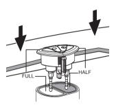
Loose Eight-square Nut and adjust the height of Rod to expected, then screw Eight-square Nut tightly.
