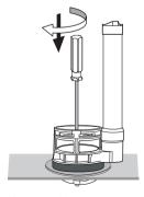
3. Use screwdriver to screw up the nut tightly.
