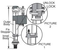
3.At the base of the fill valve's outer body, unlock the fix stopper(see picture 1)by pushing it down, then twist the outer body (see picture 2) clockwise to unlock. Adjust the outer body to the desired height. Affter setting it, twist the outer body counter clockwise to lock it to that position then pull the fix stopper upward to secure it.
