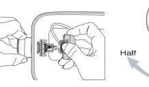
5. Important!!! Alian the grooves on the handle mechanism in vertical position (see picture).
