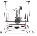
6. Fasten the tank to bowl with one pair of plastic or stainless steel bolts. Make sure bolts have the black rubber washer under
