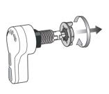
2.Unscrew the flanged nut form the handle body and rmove the square
