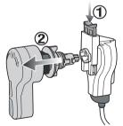
1. Push in the blue botton which is on the flush handle switch box and then pull handle out.
