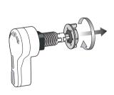
2. Unscrew the flanged nut form the handle body and rmove the square
