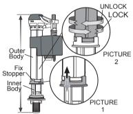
3.At the base of the fill valve's outer body, unlock the fix stopper(see picture 1)by pushing it down,then twist the outer body (see picture 2) clockwise to unlock.Adjust the outer body to the desired height.
