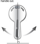
4. Make sure the handle in vertical position, it swings left and right approx. 90degress
