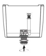
3. Insert the flush valve's base into the water tank. Screw on the nut collar and hes nut properly.
