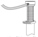
2. Connect the refill tube with refill restrictor from fill valve to the overflow pipe of the flush valve.
