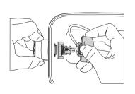
5. Important!!! Align the grooves on the handle mechanism in vertical position (see picture).
