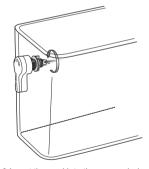
3.Insert the seal into the square hole on the water tank (fits only one way)
