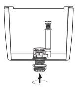
3.Insert the flush valve's base into the water tank. Screw on the nut collar and hes nut properly.
