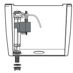
1.Insert the new fill valve with silicon seal at the base in the inlet hole of water tank and screw on the nut with collar tightly.
