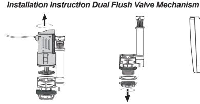
1. Hold the base of the flush valve and rotate the body counterclockwise take it out from base.
