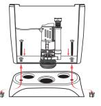
6. Fasten the tank to bowl with one pair of plastic or stainless steel bolts. Make sure bolts have the black rubber washer under
