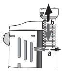
5. To adjust the height of the overflow pipe, slide the lock (a), then set the desired height of the overflow pipe(b). Put the lock back after.
