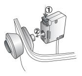
Push in switch box's green button(1) to connect with button body
