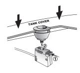
3. Push in switch box's green button(1) to connect with button body.
