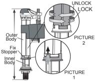
3.At the base of the fill valve's outer body, unlock the fix stopper(see picture 1)by pushing it down, then twist the outer body (see picture 2) clockwise to unlock. Adjust the outer body to the desired height. Affter setting it, twist the outer body counter clockwise to lock it to that position then pull the fix stopper upward to secure it.
