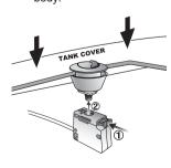
3. Push in switch box's green button(1) to connect with button body.
