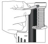
Connect the refill tube with refill restrictor from fill valve to the overflow pipe of the flush valve.
