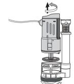
1. Hold the base of the flush valve and rotate the body counterclockwise. Take it out from base.
