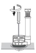
3. Use screwdriver to screw up the nut
