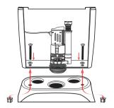
5.Insert the tank to bowl rubber gasket 6. Fasten the tank to bowl with one pair of on to the flush valve's outlet bottom. plastic or stainless steel bolts. Make sure bolts have the black rubber washer under
