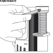
2.Connect the toilet bowl refilling tube from fill valve to the overflow pipe of flush valve.
