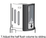
the marked part up or down.when the buoy is higher the discharge water volume
