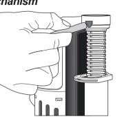
2.Connect the toilet bowl refilling tube from fill valve to the overflow pipe of flush valve.
