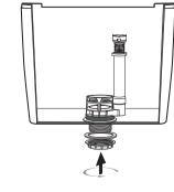
3.Insert the flush valve's base into the water tank.Screw on the nut collar and hes nut properly.
