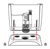
6. Fasten the tank to bowl with one pair of plastic or stainless steel bolts. Make sure bolts have the black rubber washer under the bolt's head.
