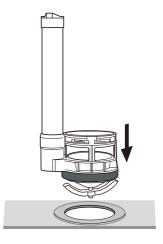
2.Put the base into the ceramic hole.
