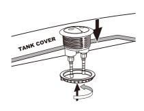
3. Put the body of button into the hole tighten the nut.
