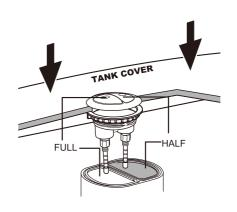
4. Install the tank cover into the tank.
