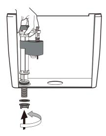
1.Insert the new fill valve with silicon seal at the base into the inlet hole of water tank and screw on the nut with collar tightly. Caution!!! Do not over tighten nut.
