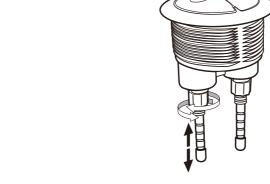
2. Loosen the adjustable nut. Adjust the rod to proper length and then fasten it.
