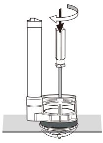
3. Use screwdriver to screw up the nut tightly.
