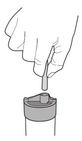
2.Connect the toilet bowl refilling tube from fill valve to the overflow pipe of flush valve.
