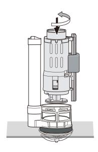
4. Screw up the body of the flush valve clockwise.
