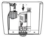
4. Take the body of flush valve and set it into the base and lock in place by rotating it clockwise.
