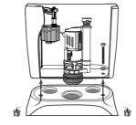
6. Take the water tank and install it on the two piece toilet of mounting holes, then fasten the bolts.
