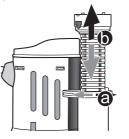
9. To adjust the height of the overflow pipe, slide the lock (a), then set the desired height of the overflow pipe(b). Put the lock back after.
