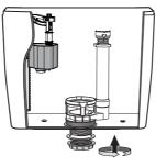
3. Adjust the screw to adjust the water
